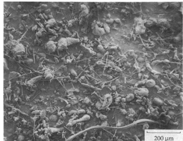
Figure 12 Scanning electron micrograph of 5 vol % composite with Saffil bulk (run AB2) after 10 min ball milling.
