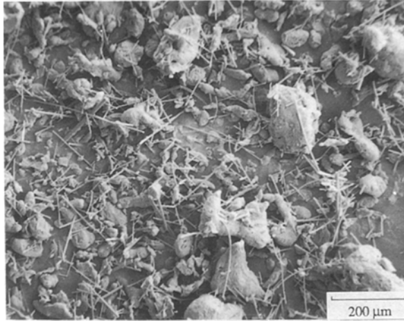
Figure 17 Scanning electron micrograph of 5 vol % composite with Saffil milled RF590 (run AM2) after 5 min ball milling.
