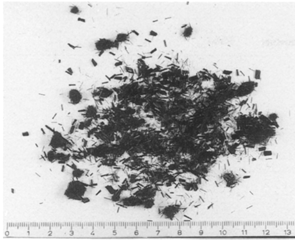
Figure 5 Nicalon SiC fibres in as-received condition. Note primary multifilament chops and secondary clusters.
