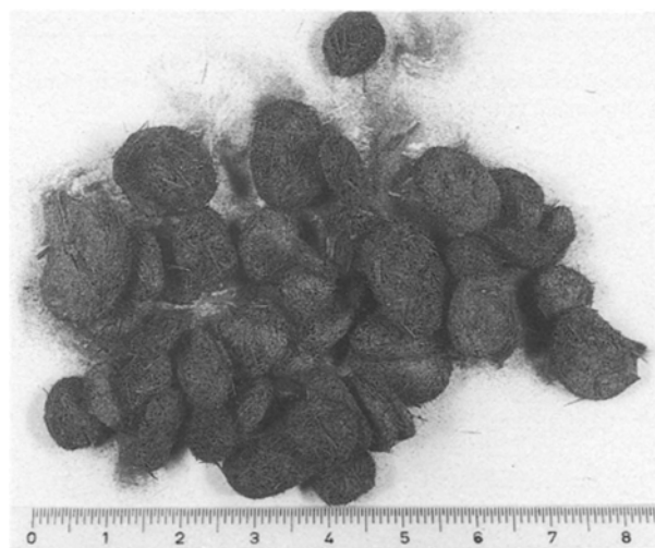
Figure 8 Large, compact and oblate clusters of Nicalon SiC fibre as obtained after milling (run S2). Note that the fraction of fibres shown is not representative for the actual volumetric composition.
